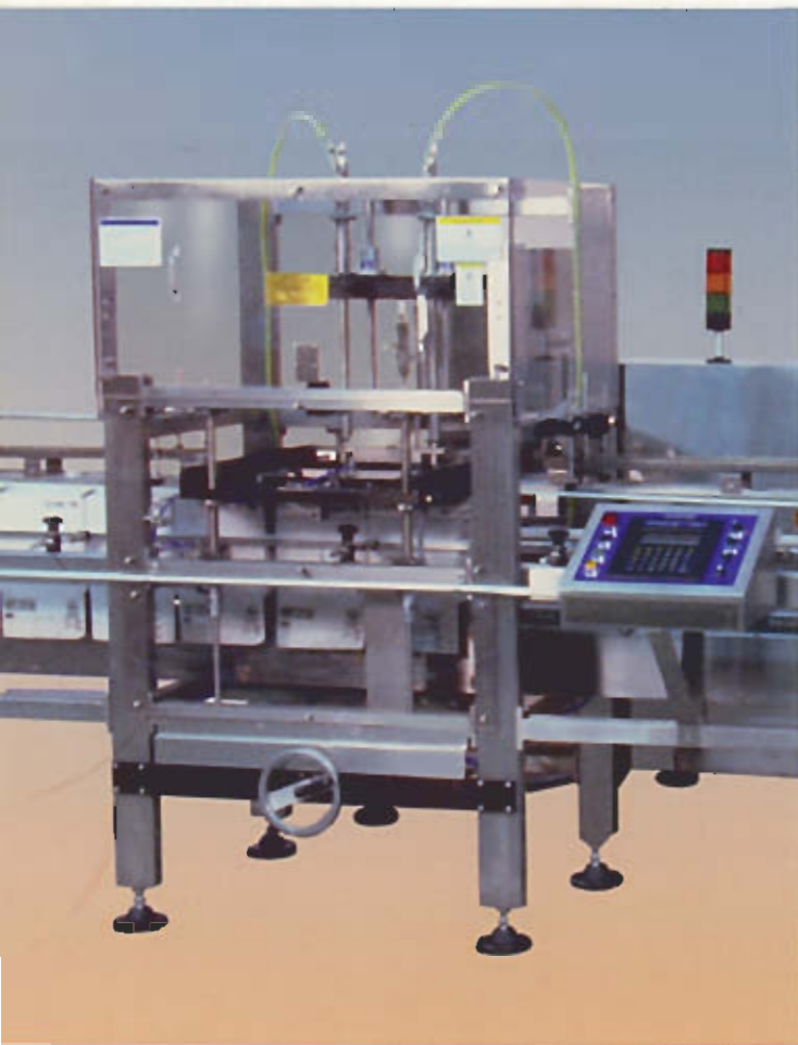
The filler handles container sizes from 10 to 20 liters, at production rates from 4 to 10 containers per minute.
